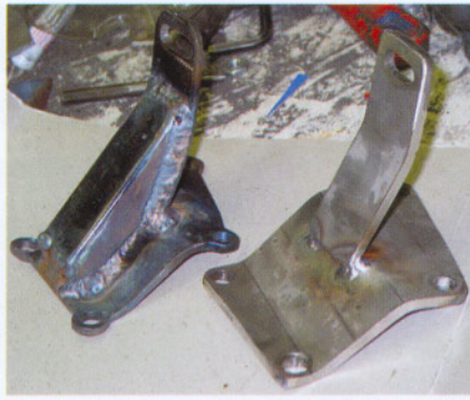
Above: Six-speed CGR gearbox (top) is 15mm shorter than the five-speed. Above centre: First job was to fabricate new gearbox mountings. This picture shows Patrick Carlier's 'prototype' (left) and the final stainless steel version. Above right: All the six-speed parts needed arrived in a box from Patrick. Right: Milling the spacer to take up the gap between the propshaft coupling and the gearbox. Below: The old five-speed shift rod.
