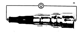
Connector resistance should be 4000 to 6000 ohms.
