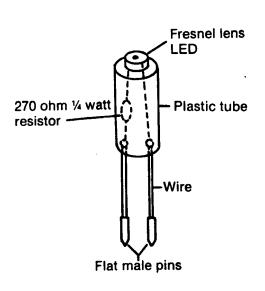
An LED is used to check the low voltage signal from the reference mark and speed sensors. One of these testers will be sent to every dealer. The tester, however can be made from locally available components which are available at Radio Shack or any other electronics store.
