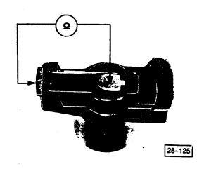
Rotor resistance should be about 1000 ohms.
