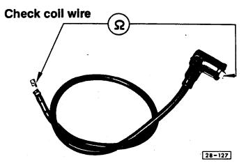
Coil wire resistance should be 800 to 1200 ohms.
